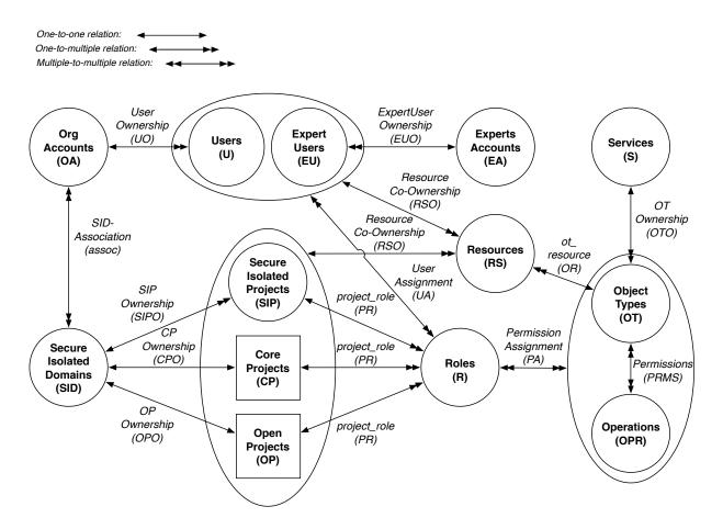
Figure 3.1: Secure Isolated Domain Model (SID-model)
