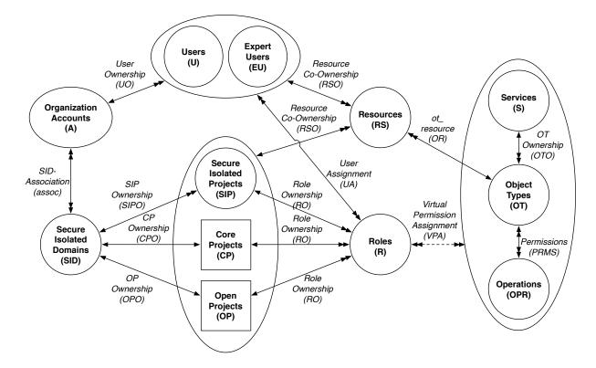
Figure 5.3: AWS Access Control Model with SID Extension (AWS-AC-SID)
