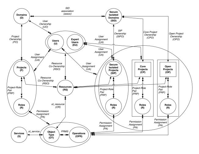
Figure 4.8: OpenStack Access Control Model with SID Extension (OSAC-SID)
