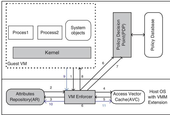
**Figure 4: Our VMM-based OS Kernel Integrity Protection Architecture**
