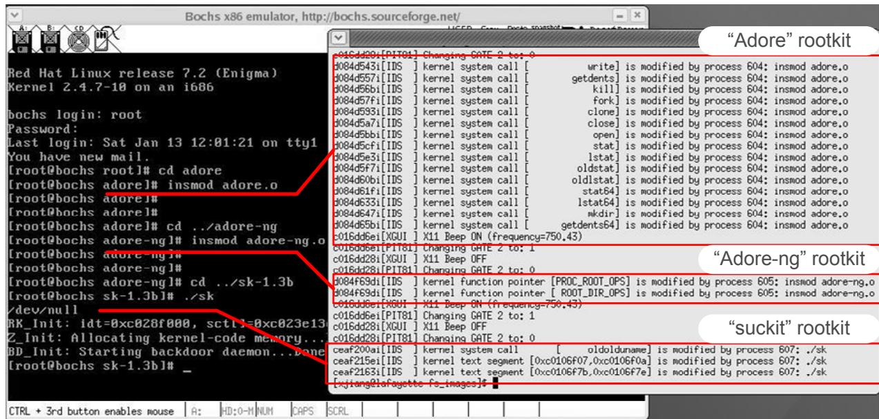
Figure 6: Detecting and preventing OS kernel integrity violations
