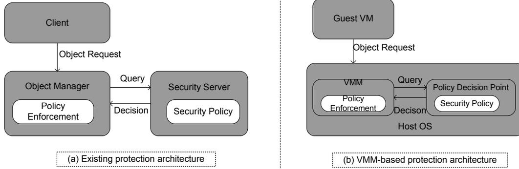
**Figure 1: Existing protection architecture (within the same OS) vs. our VMM-based protection architecture**
