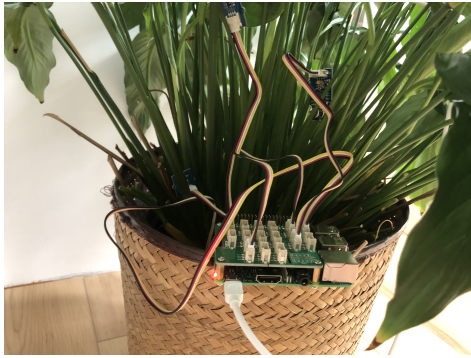
Fig. 2. Indoor plant remote monitoring IoT setup.
