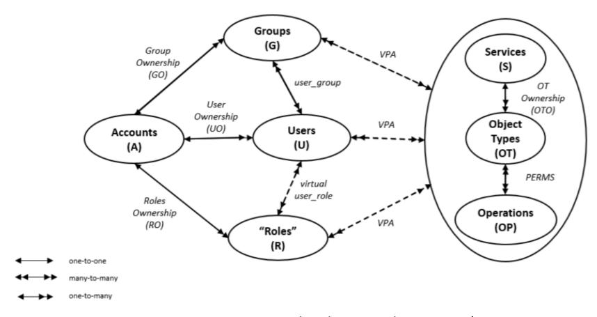
Fig 1: AWS Access Control within a Single Account \*
