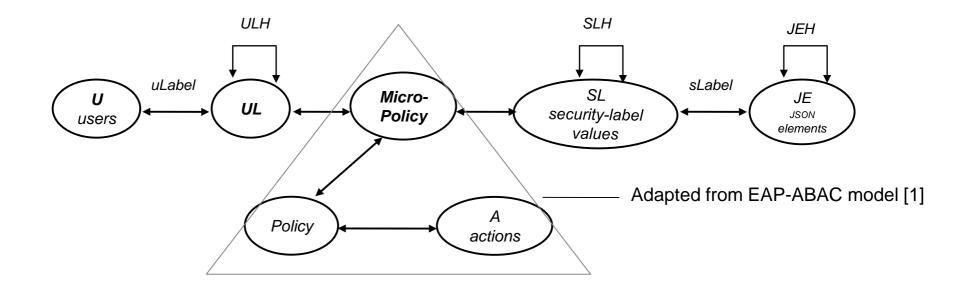
Fig 4: The Attribute-based Operational Model (AtOM)
