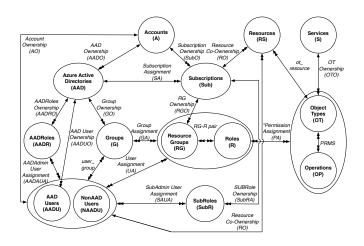
Figure 1: Azure Access Control (Azure-AC) Model
