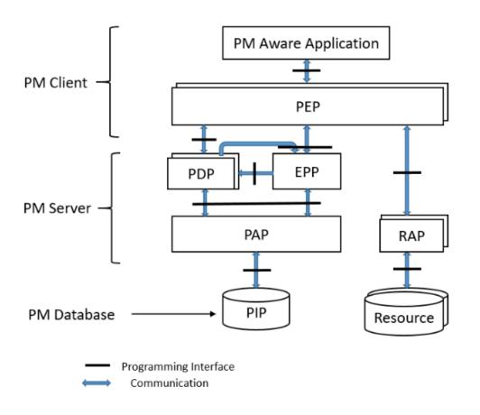
Fig 5. Architectural Components of PM Adapted from [\*]
