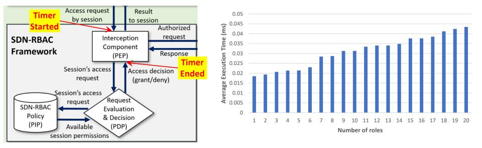
Average execution time required by SDN-RBAC components to finish checking 50 operations with varying number of roles.
